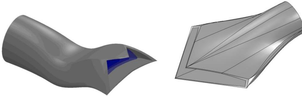
**Figure 4: Inlet and tailpipe**
