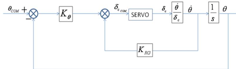
Figure 14: Pitch control loop
