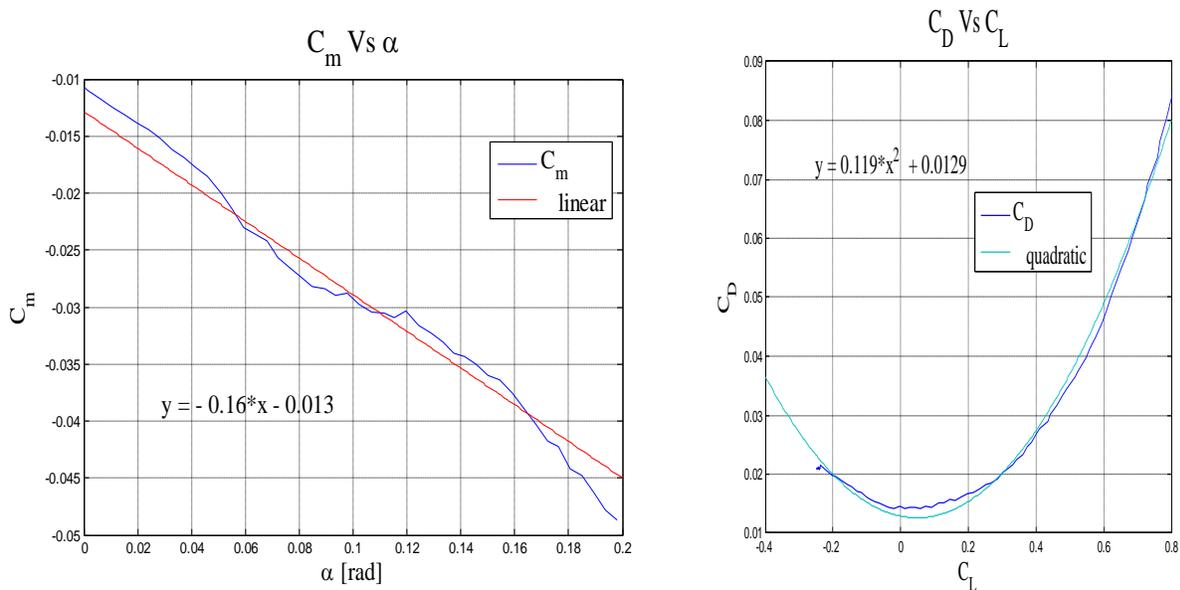
Figure 10: Wind tunnel test results – longitudinal plane
