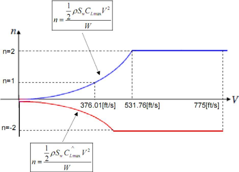
Figure 12: V-N diagram
