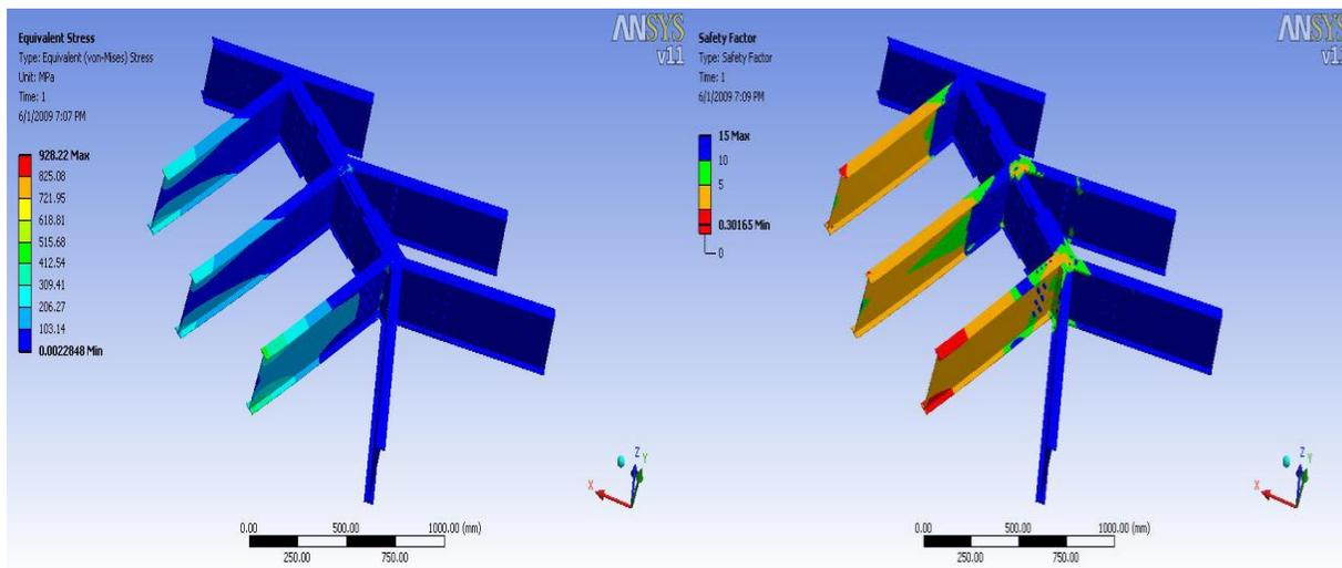
**Figure 8: Beam connection Ansys results (left: VM stress, right: safety factor)**
