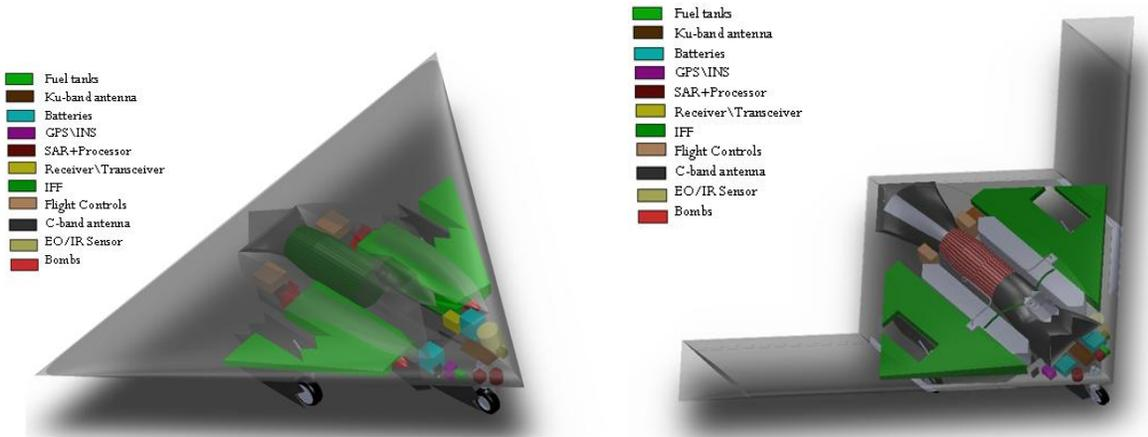
**Figure 3: Layout of both configurations**
