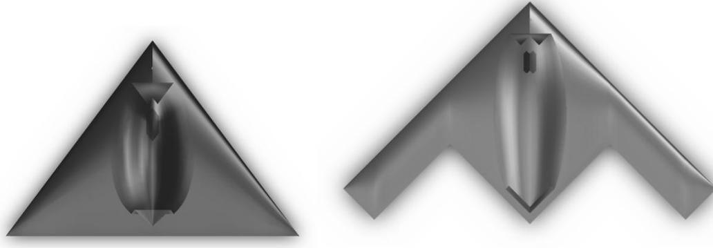
**Figure 2: Delta wing (left) and lambda (right)**
