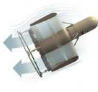
Air flows through duct, providing lift and control
