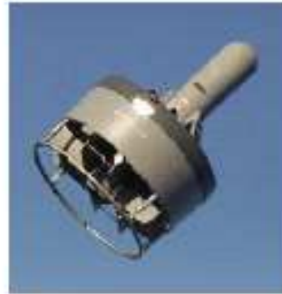
Air flows through duct, providing lift and control
