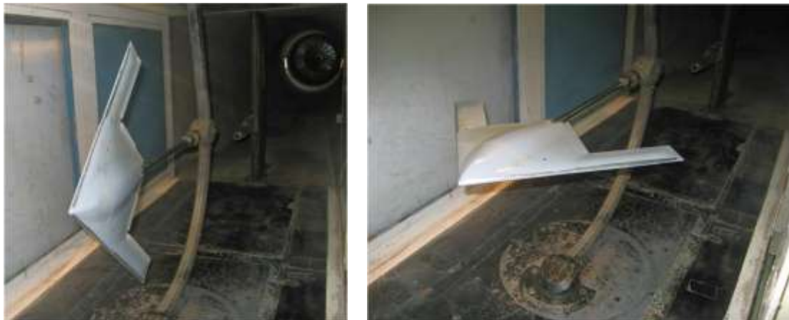
Figure 12: Model mounted in the wind tunnel for pitch (left) and yaw (right) measurements.
